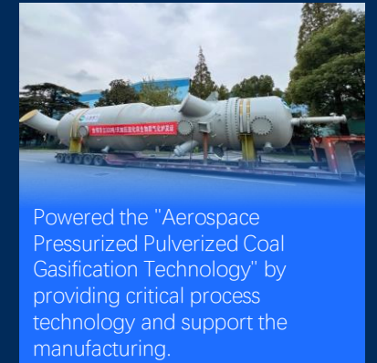
World's first 300 TPD pure oxygen pressurized fluidized bed biomass gasifier.
